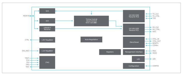
Fig 1. 88E1116R Functional Block Diagram
