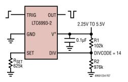
Figure 7. 100µs Negative Pulse Generator
