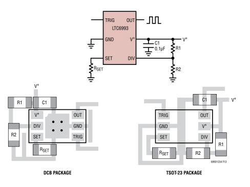
Figure 13. Supply Bypassing and PCB Layout
