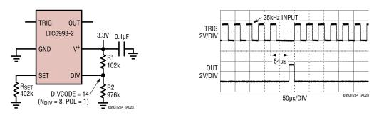
Use retriggerable one shot with output inverted. Output remains low as long as retrigger occurs within t<sub>OUT</sub> = 64µs.
