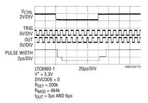
Figure 10. Typical Settling Time
