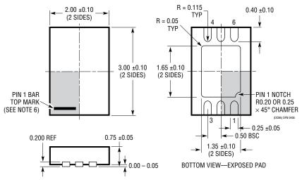
DCB Package 6-Lead Plastic DFN (2mm × 3mm) (Reference LTC DWG # 05-08-1715 Rev A)
