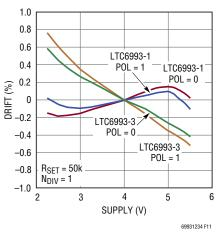
Figure 11. t<sub>OUT</sub> Drift vs Supply Voltage
