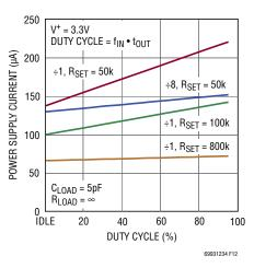
Figure 12. I<sub>S(ACTIVE)</sub> vs Output Duty Cycle
