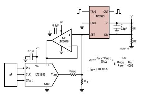
Figure 9. Digitally Controlled Pulse Width
