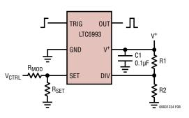
Figure 8. Voltage-Controlled Pulse Width
