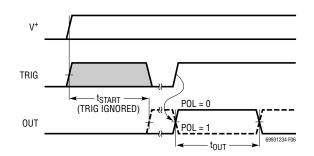
Figure 6. Start-Up Timing Diagram
