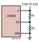
Figure 1. Simple Technique for Setting DIVCODE
