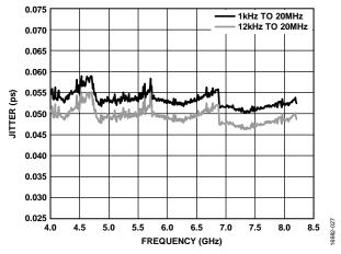
Figure 27. RMS Jitter, Fractional-N,  $f_{PFD} = 153.6 \text{ MHz}$ ,  $VCC\_VCO = 5 \text{ V}$
