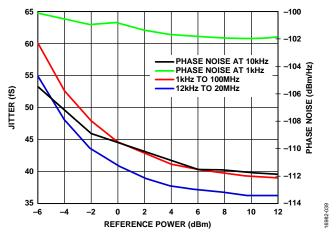
Figure 33. Jitter and Phase Noise,  $f_{PFD} = 250 \text{ MHz}$
