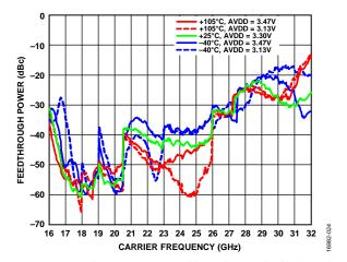
Figure 24. RF32P and RF32N VCO × 3 Feedthrough, De-Embedded Board and Cable Measurement, Combined Using Balun
