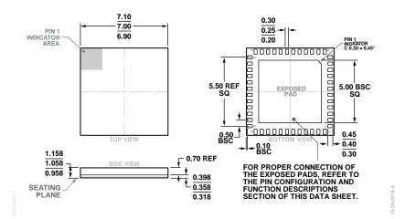
Figure 45. 48-Terminal Land Grid Array [LGA] (CC-48-4) Dimensions shown in millimeters
