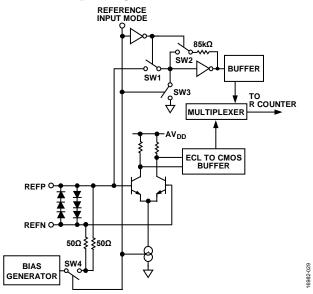
Figure 35. Reference Input Stage, Differential Mode
