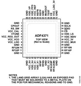
Figure 6. Pin Configuration
