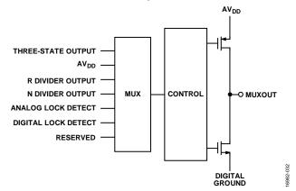
Figure 38. MUXOUT Schematic
