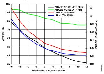
Figure 34. Jitter and Phase Noise,  $f_{PFD} = 100 \, \text{MHz}$
