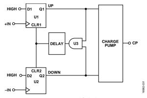
Figure 37. PFD Simplified Schematic
